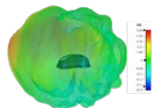
3D Plot Element 2 Side (5400 MHz)
