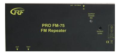
There is only one adjustm3ent in the PRO FM-75 repeater. OUTPUT LEVEL should be adjusted as the output power level indicator LED turns from green to red. Then the gain should be reduced as much as the LED turns just green. If LED lights as double color red/green as almost orange is the output level near to change to too high.
