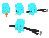
Make sure the cables are slotted facing left and right as shown below.
