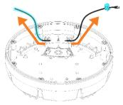
Insert the glands on the slots respectfully leaving a sufficient cable length to be able to connect the router.
