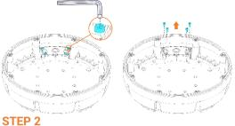
Open the cap that has a silicone strap attached to it.
