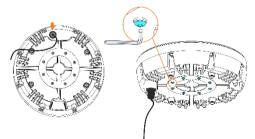
• Align the ethernet cable on the paths engraved on the antenna base.
