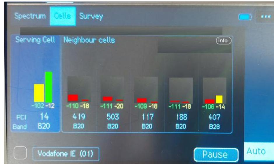
Rotate the Yagi antenna slowly through 360 degrees, and note the different Cells that become the Serving cell.
