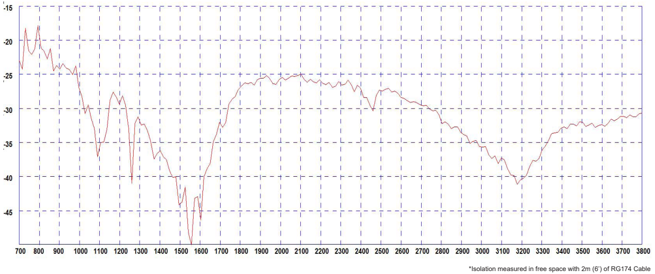
Typical Isolation Elements 1&2*
