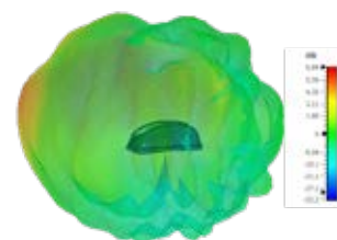
3D Plot Element 2 Side (5400 MHz)
