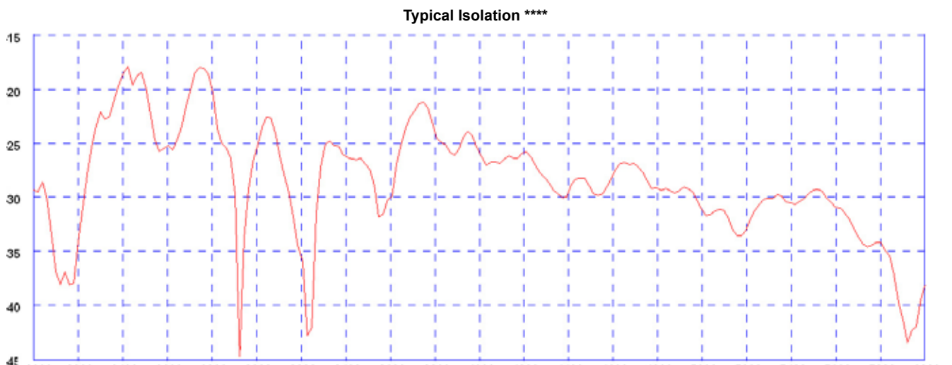
****Typical worst case isolation measured on a 600x600mm (2'x2') ground plane without cable loss
