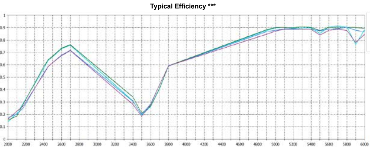
***Efficiency simulated in CST Microwave Studio for each element fed without cable loss on 600x600mm (2'x2') ground plane
